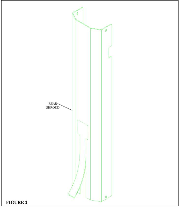
• If the 663101 SECOND STACK OPTION is not installed, the rear SHROUD opening must be removed. Apply pressure to the bottom of the SHROUD where the "V" groove is and carefuly remove the weight stack opening on the SHROUD as shown in FIGURE 2.
